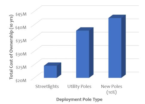
The savings can be even bigger if new utility poles must be erected, due to lack of adequate pole infrastructure in a key location. We considered one case in which 10% of repeater sites could not be served by utility poles, and needed a new pole. In our home city of San Jose, we believe that 10% is a conservative figure... the number of new poles could be much higher.
